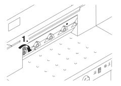
Push in the first screw on the left side and tighten.
