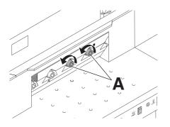
Loosen slightly screws (A) so that the blade slides onto the cutting stick.
