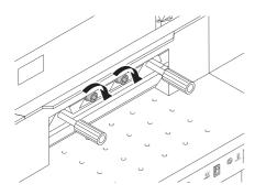
Screw in middle screws and tighten.
