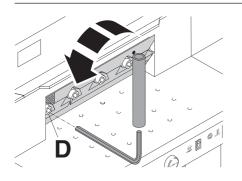
Remove the left screw  $(\mathbf{D})$ , using the extension.
