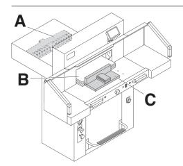
Position the paper on the backgauge (**A**) and side lays left or right (**B**). To move paper stacks, please use the paper knock-up block (**C**) provided. (Run backgauge to the front for turning the paper stack).
