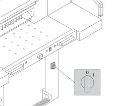
Replacement of blade and cutting stick may be performed only when the main switch is switched off!
