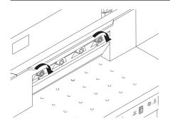
Slightly screw in outer screws.
