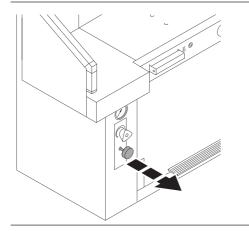
Pull out blade locking key  $\rightarrow$  blade moves to the top.
