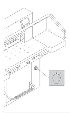
When not in use for a longer period switch off. (Main switch to " $\mathbf{0}$ ").
