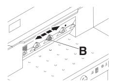
Push the blade and screw (**B**) as far as possible to the left or right and then centralize them.  $\rightarrow$  The blade must rest on the cutting stick.
