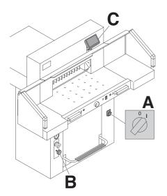
Display (C) is pivotable. By loosing the allen head screw (D), (allen wrench is in the tool box) the display can be pivoted within the elongated hole. Tighten allen screw again.
