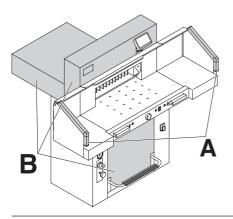
All components which could endanger the operator are covered by a guard (**B**)!
