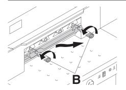
Simultaneously slightly loosen both screws (**B**) and remove blade with blade changing tool.
