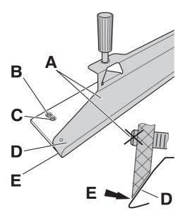
Take the exchange blade carefully out of the blade box and screw it to the blade changing tool (D).
