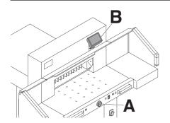
The measurement is set either with the handwheel (**A**) or by programming (**B**) the cutting measurements. Measurement is shown on the display in inches or cm (**B**).
