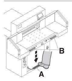
The clamp moves automatically when cutting is activated. The paper can be pressed in advance, with the foot pedal (**A**). Cutting is activated by pressing both buttons (**B**) on the front table.
