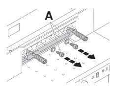
Remove remaining two screws (A).
