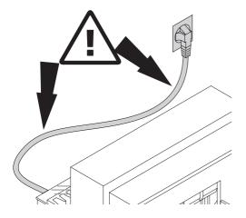
Protect mains cable against heat, oil and sharp edges!
