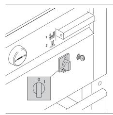
Replacement of blade and cutting stick may be performed only when the main switch is switched off!
