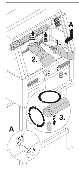
Take out the cutting stick with a small screwdriver. If needed the cutting stick can be turned or exchanged. (The cutting stick can be used eight times).
