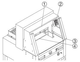
After 30 minutes the machine (1) (2) (3) (4) switches to energy-saving mode. The machine is reactivated by touching the keypad area 12.
