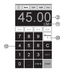
How to program Memory 3 and 4 Press the memory button (29) to enter the memory platform (3 or 4). Enter the required measurements or overwrite them. Press the button and keep it pressed until an acoustic signal sounds, the measurements have been saved now.
