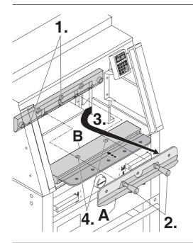
Remove 2 blade screws 4860 and 3 blade screws 5260, 6660 (1.). Loosen the grips (2.) of the blade changing tool (A) lightly and allow the blade to be taken downwards out of the machine (3.). Place the blade into the blade carrier (B) and screw it into place (4).
