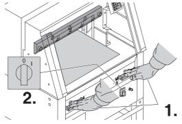
Lower the blade by pressing both cutting buttons (1.). Keep one button pressed and turn off the main switch (2.).
