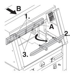
Lightly tighten 3 (4860 has 2) of the 5 blade screws with washers (1.). Remove the blade changing tool (2.). Lightly tighten the remaining blade screws with washers (3.). Return blade changing tool to tool holder (B).
